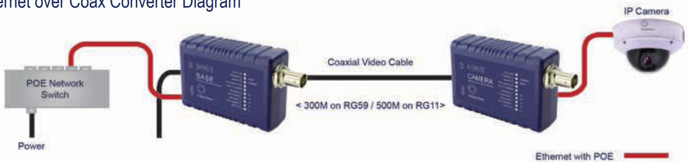
Diagram 1. Ethernet over Coax Converter delivers Ethernet and POE over legacy coax, for maximum reliability with minimal wiring.
